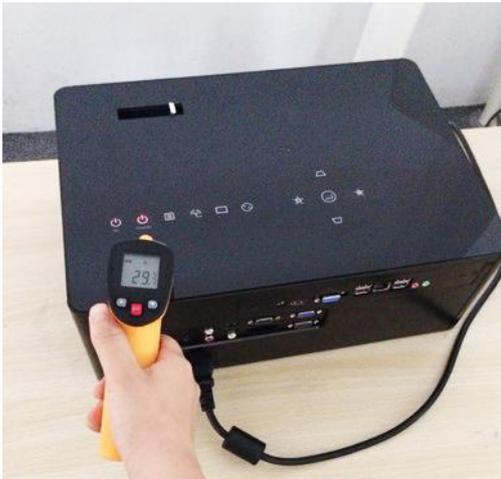
Perfect internal design with aluminum shell which brings very powerful radiation function. The temperature of the device is 33°C when it's running, compare with some projector, the temperature is 10°C lower.
